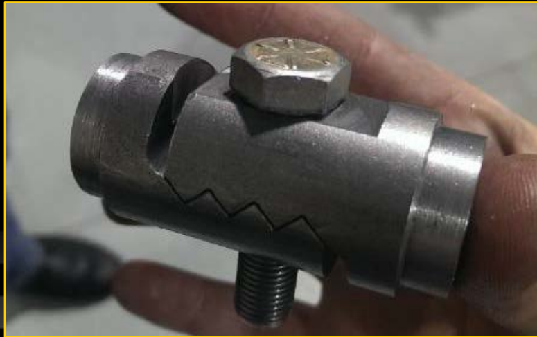
Fig 3: Assembled ruffle chip tube inserts
